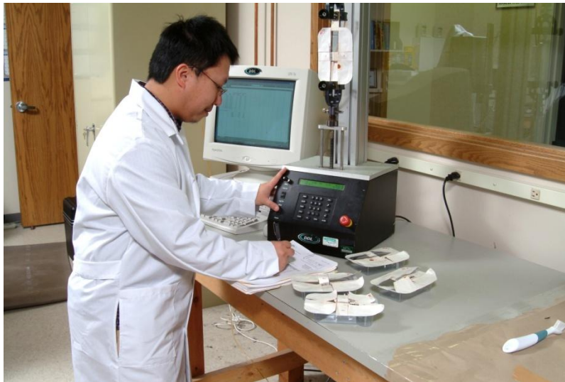
Seal Strength Testing per ASTM F88
