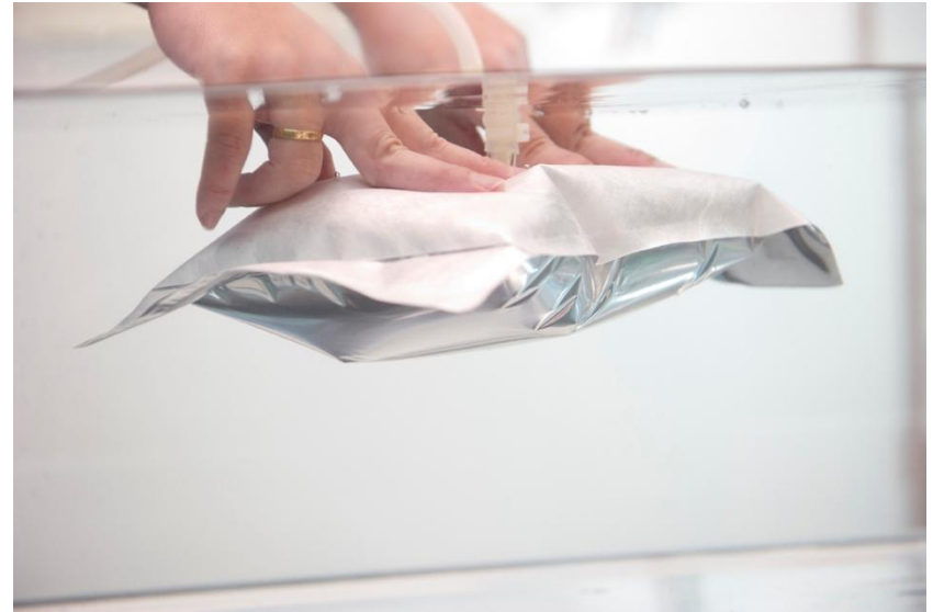
Bubble Leak Testing per ASTM F 2096
